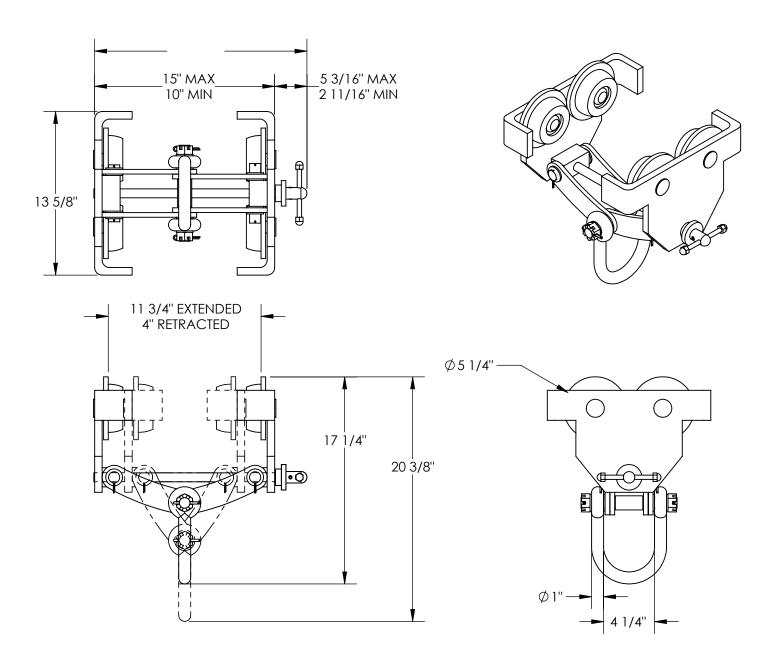
MODEL NUMBER IS SMS-09-V46-QIT-8 FITS BEAM FLANGE WIDTH OF 4" TO 11 3/4" HEADROOM IS 13 7/8" OVERALL WIDTH IS 20 3/16" OVERALL LENGTH IS 13 5/8" OVERALL HEIGHT IS 20 3/8" MAX AND 17 1/4" MIN UNIFORM CAPACITY LOAD IS 8,000 LBS STEEL CONSTRUCTION WITH PAINTED FINISH 4 1/4" SHACKLE
