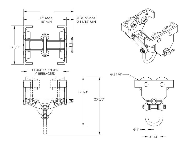
MODEL NUMBER IS SMS-09-V46-QIT-10 FITS BEAM FLANGE WIDTH OF 4" TO 11 3/4" HEADROOM IS 13 7/8" OVERALL WIDTH IS 20 3/16" OVERALL LENGTH IS 13 5/8" OVERALL HEIGHT IS 20 3/8" MAX AND 17 1/4" MIN UNIFORM CAPACITY LOAD IS 10,000 LBS STEEL CONSTRUCTION WITH PAINTED FINISH 4 1/4" SHACKLE
