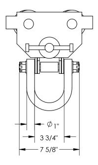
MODEL NUMBER IS SMS-09-V46-QIT-6 FITS BEAM FLANGE OF 3" TO 7 1/2" HEADROOM IS 10 3/8" OVERALL WIDTH IS 16 7/8" OVERALL LENGTH IS 11" OVERALL HEIGHT IS 14 9/16" MAX TO 12 3/8" MIN UNIFORM CAPACITY IS 6,000 LBS. STEEL CONSTRUCTION WITH PAINTED FINISH 3 3/4" SHACKLE
