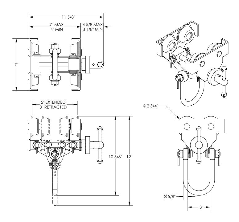
MODEL NUMBER IS SMS-09-V46-QIT-2 FITS BEAM FLANGE OF 3" TO 5" HEADROOM IS 8 1/8" OVERALL WIDTH IS 11 5/8" OVERALL LENGTH IS 7" OVERALL HEIGHT IS 12" MAX TO 10 5/8" MIN UNIFORM CAPACITY IS 2,000 LBS STEEL CONSTRUCTION WITH PAINTED FINISH 3" SHACKLE
