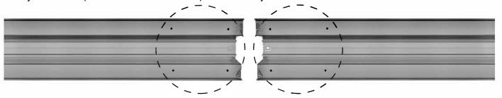
2 Insert the cover screw and nut as shown in picture, tighten. Then turn track upside down exposing the 4 hole pattern. Do this on both tracks, only on the ends to be joined together.
