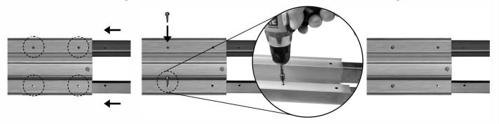
4 Slide the second track onto the connector angles. Make sure the parts are on a flat surface and that they fit tightly together. Then drill in two self tapping screws on the opposite end. When all four outside screws are secure drill in the 4 center screws.
