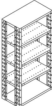
Stand unit up. Dura-Tech frames DO NOT require any bracing. Use a large handled screwdriver to tighten bolts for maximum tightness.
