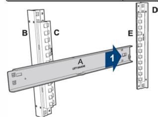
Insert the rear hook of the rail into the rectangular slot of the rear mounting bracket.
