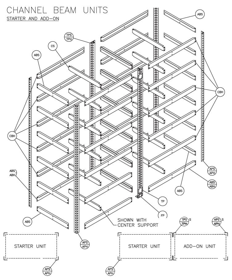
NOTE: WHEN ORDERING CHANNEL BEAM UNITS, ALL BOTTOM LEVEL BEAMS AND ALL FRONT-TO-BACK BEAMS ARE STANDARD ABS ANGLE BEAMS.
