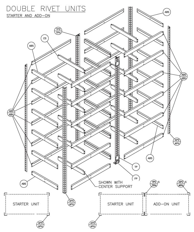
NOTE: WHEN ORDERING HEAVY-DUTY-ANGLE BEAMS UNITS, FRONT TO BACK BEAMS ARE
