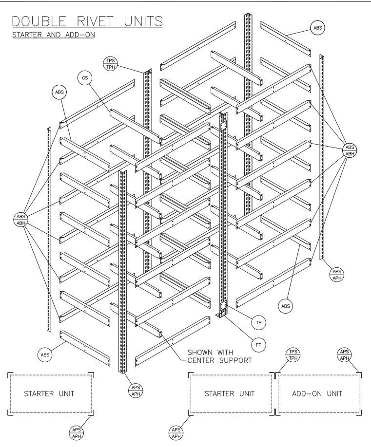
NOTE: WHEN ORDERING HEAVY-DUTY-ANGLE BEAMS UNITS, FRONT TO BACK BEAMS ARE STANDARD ABS BEAMS.
