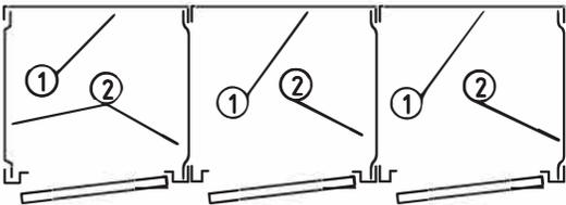
SIDE PANELS MUST GO INSIDE REAR PANEL AND INSIDE FRAME.
