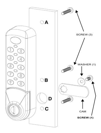
Attach lock to locker door with three screws.
